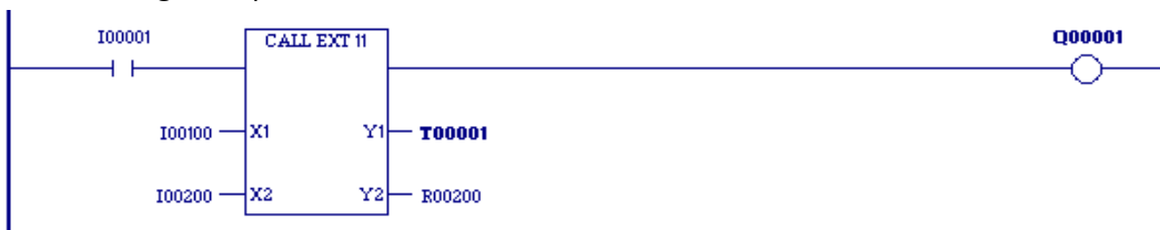
Figure 7: Calling an External Block in Ladder Logic
